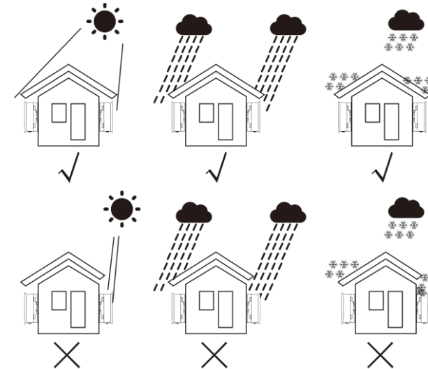
Figure 5.1 Recommended Installation locations
