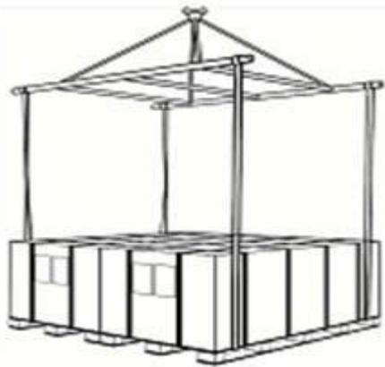
Use reasonable hoisting jigs, hoisting allows up to 2 supporting modules at a time. Before hoisting, confirm whether the pallets and cartons are damaged and whether the hoisting ropes are strong and firm. When the hoisting is about to touch the ground, two of them will straighten the carton and gently place it on a relatively flat position
